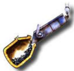
Adding steel scrap
